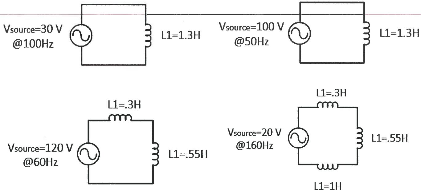
2. Solve for total current in the following circuits and for the voltages across each inductor and resistor :
